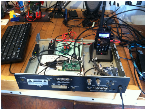
APRS Mark II Raspberry PI & Boefeng HT mounted on discarded chassis
